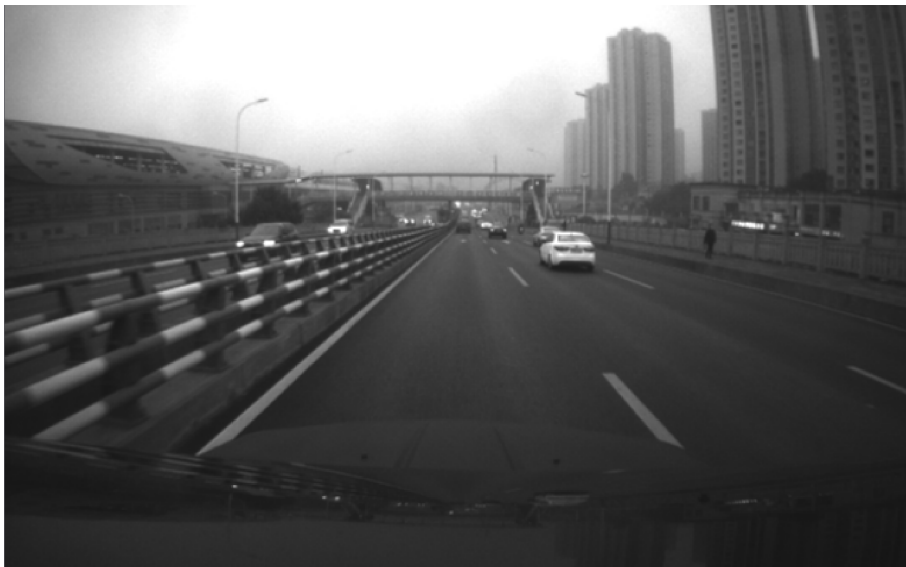
Figure 4.1.: The hood covers almost a third of the frame, preventing feature acquisition.
