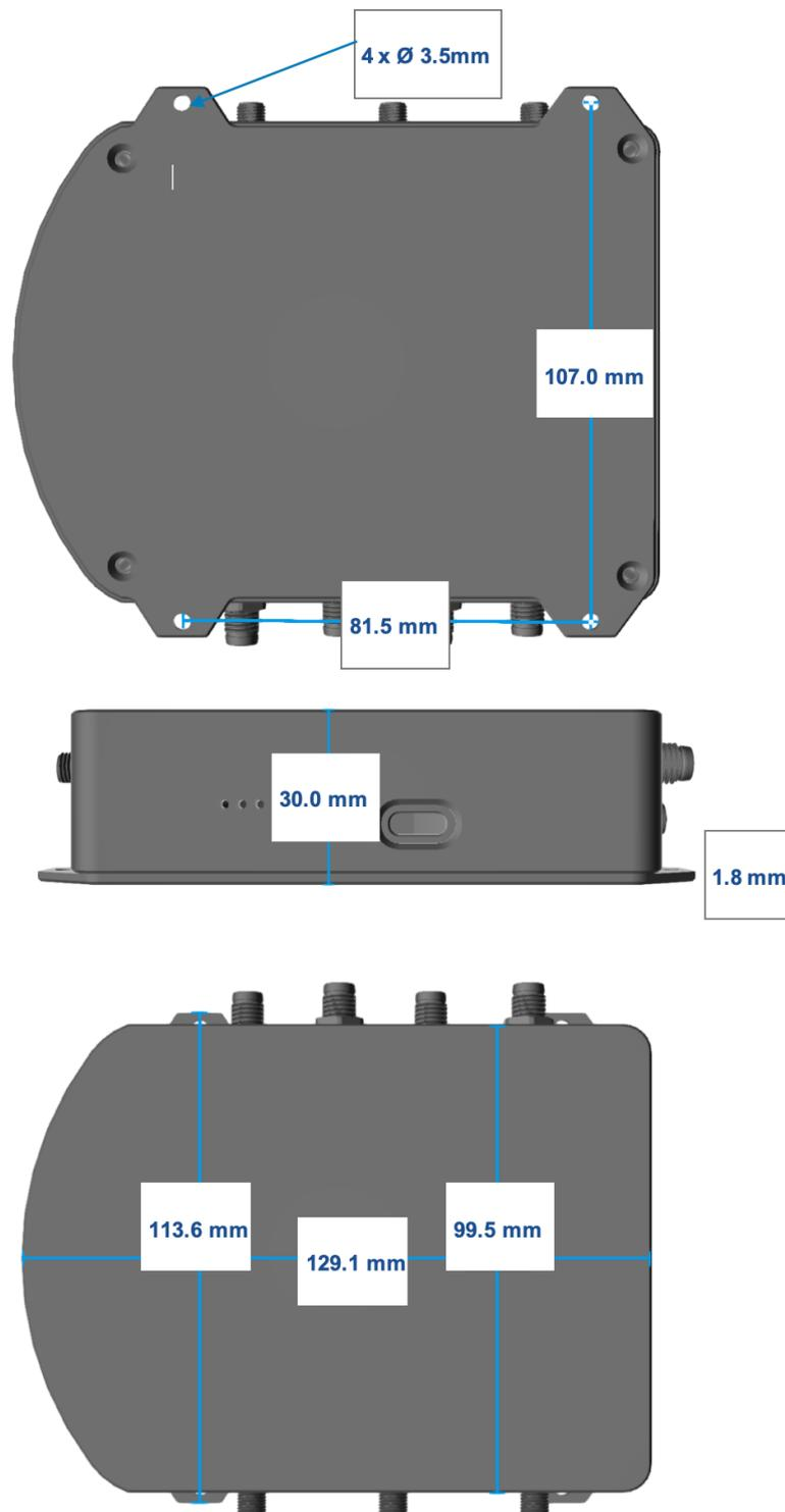
Figure 3.8.: Dimensions of the Vision-RTK 2's enclosure
