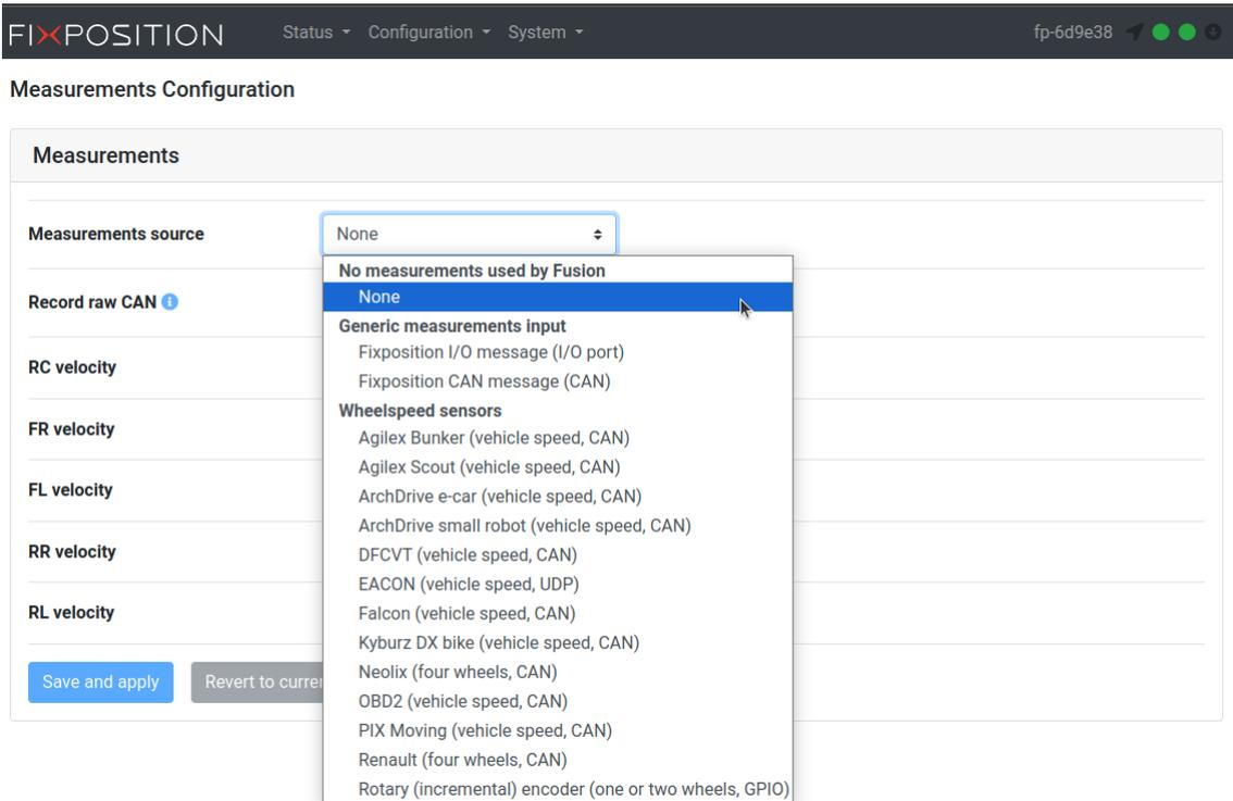
Figure 5.33.: Preset list of the CAN and I/O wheelspeed configurations
