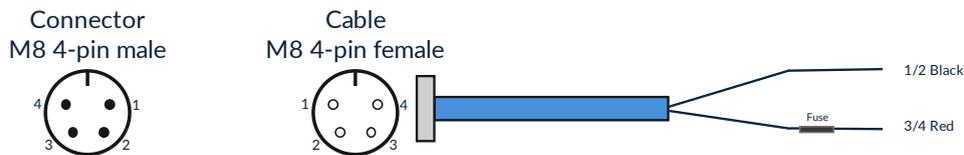
Figure 3.5.: Power connector pin overview
