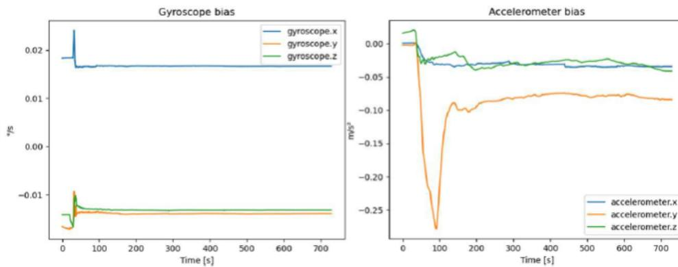
Figure 6.7.: Gyroscope and accelerometer biases over time
