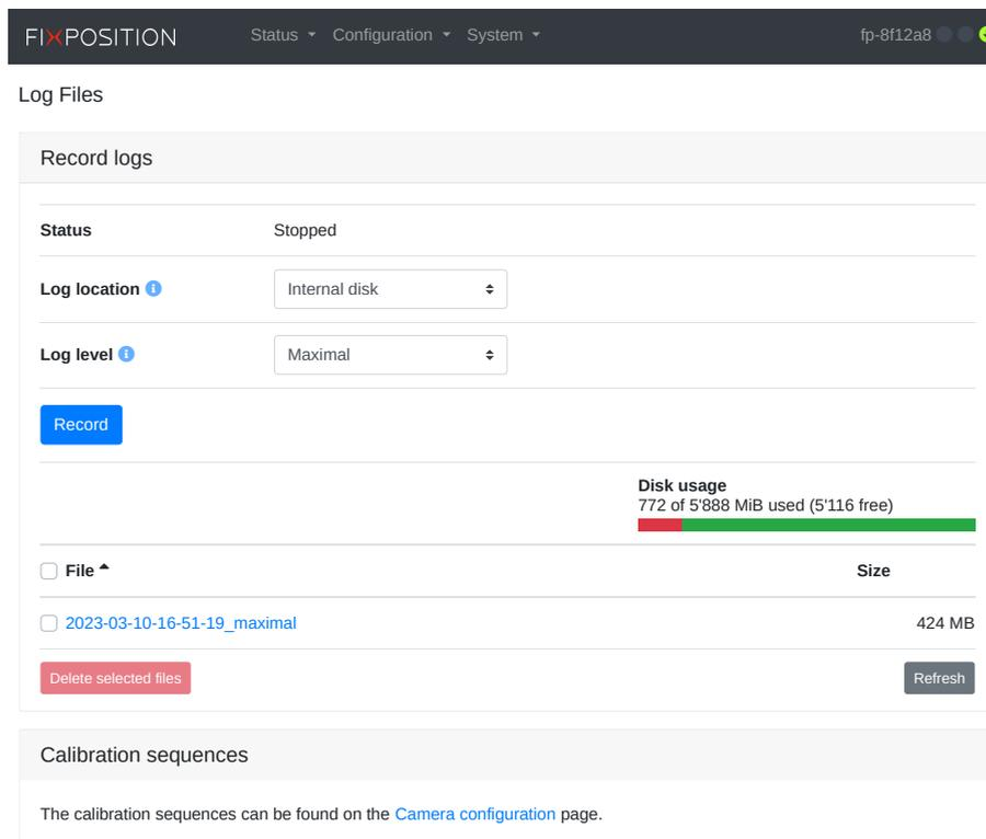
Figure 7.1.: Record data panel on the web interface
