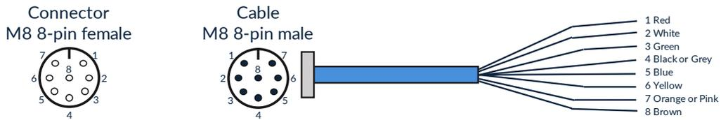
Figure 3.3.: I/O connector pin overview
