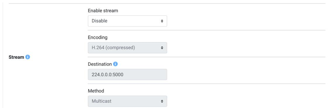
Figure 5.31.: Camera stream configuration
