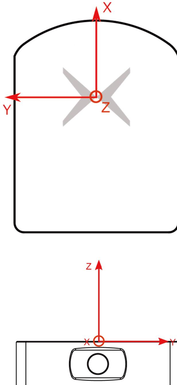
Figure 3.6.: Reference frame of the Vision-RTK 2
