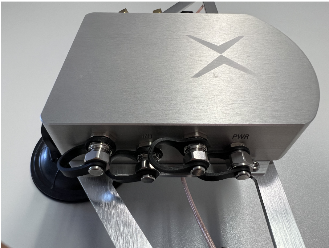
Figure 4.5.: Vision-RTK 2's connectors secured with protective caps
