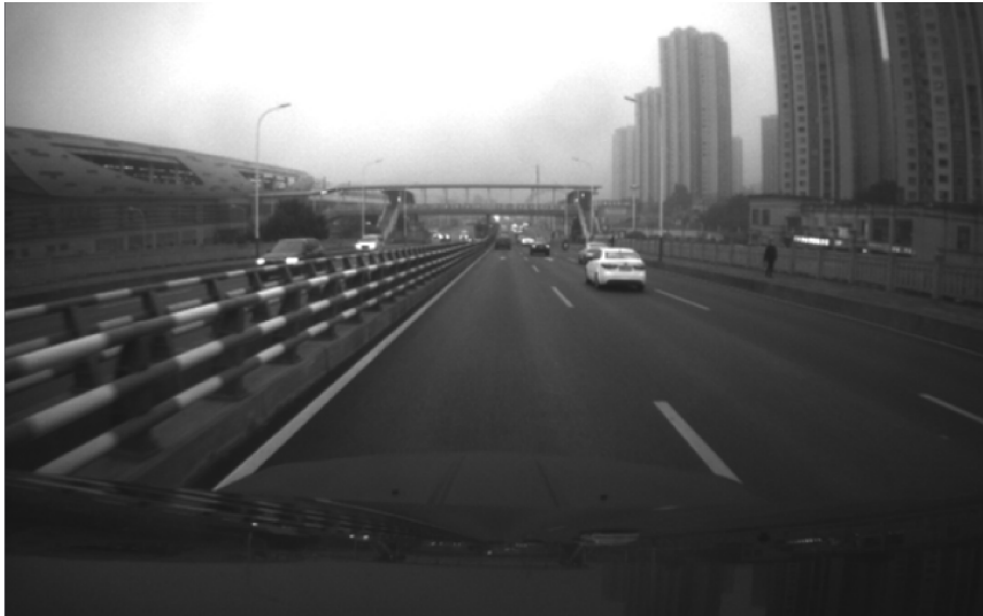
Figure 4.2.: The hood covers almost a third of the frame, preventing feature acquisition.
