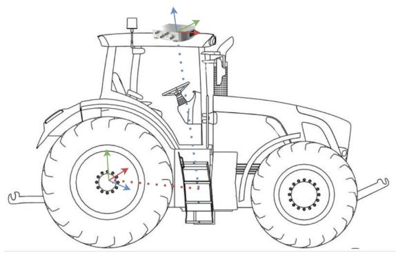
Figure 5.30.: Transform from the VRTK2's body to the output reference frame
