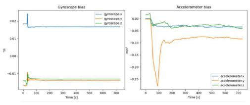
Figure 5.28.: Gyroscope and accelerometer biases over time
