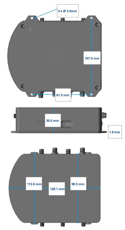
Figure 3.8.: Dimensions of the Vision-RTK 2's enclosure
