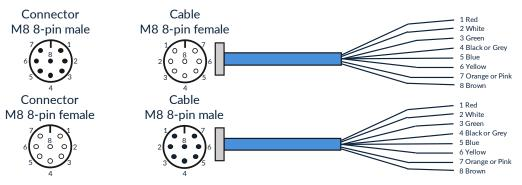
Figure 3.4.: AUX connector pin overview
