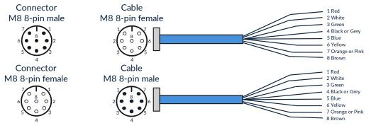
Figure 3.3.: I/O connector pin overview
