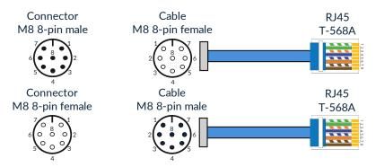
Figure 3.2.: Ethernet connector standard
