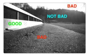
(a) Ground robot: The horizon line lies in the middle of the camera frame.
