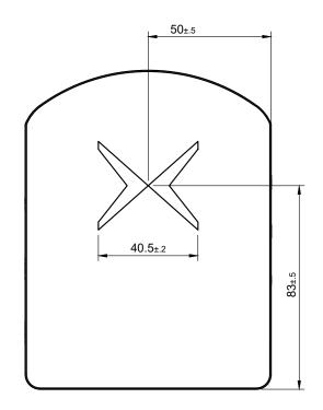
Figure 3.7.: Fixposition logo position on the Vision-RTK 2
