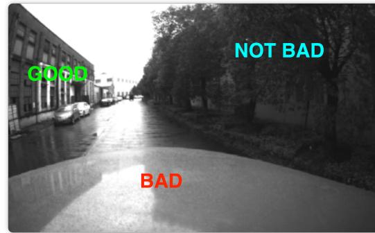
(b) Car: The hood covers almost half of the frame, preventing feature acquisition.
